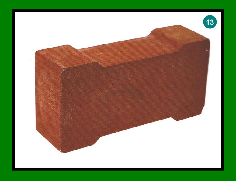
A sludge-ash brick: made entirely from dehydrated sewer sludge. The bricks are pressed in a mould and heated to 1,000 °C to burn off all organic matter.
