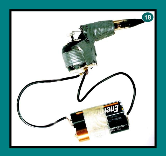
Tattoo gun: made from guitar string, a propelling pencil, a motor from a personal stereo & batteries. Ink is made by burning black chess pieces or carbon paper and mixing the ash with water.
